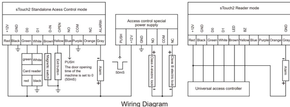
Note: Type A Electronic lock refers to the electric unlock when power on, such as electric control lock, electric lock. Type B Electronic lock refers to the electric unlock when power off, such as magnetic lock, electric bolt lock.
